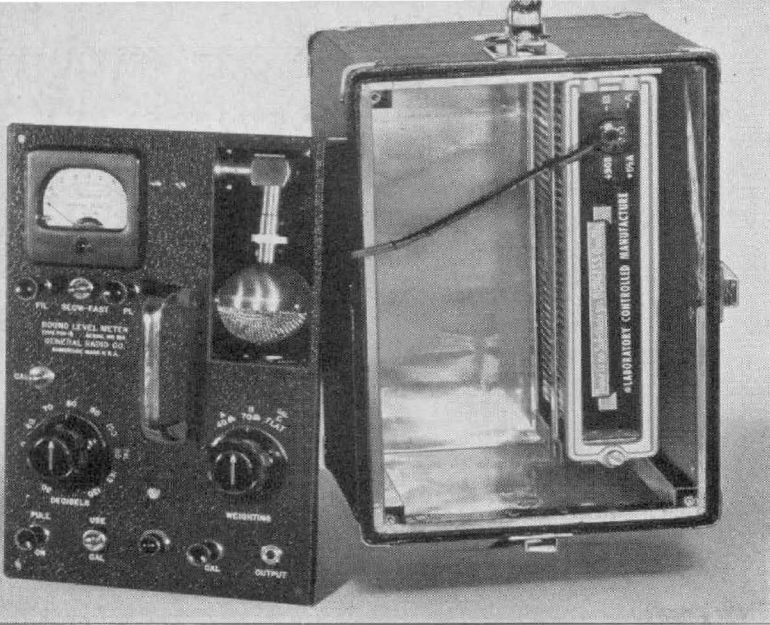
FIGURE 2. The power supply for the sound-level meter is a single block battery which mounts inside the cabinet. Connections are made with a plug as shown.
